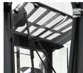
Front screen and roof with wiper / washer
